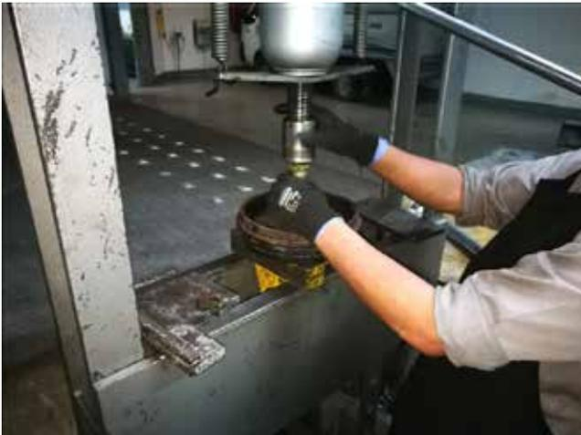
Unlike 1st gen bearings, this bearing type only needs to be manually slid and correctly aligned.
